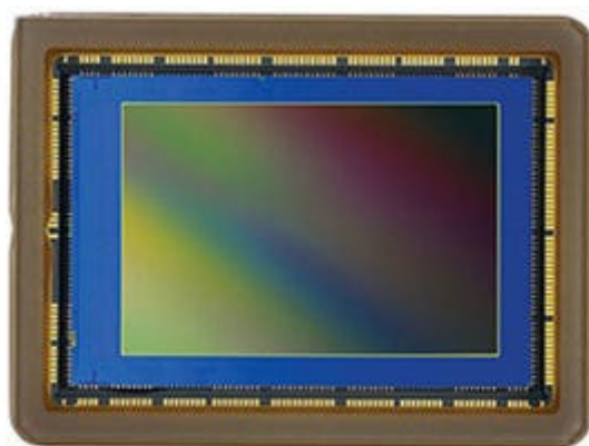
24.2 Megapixel (APS-C) CMOS Sensor
